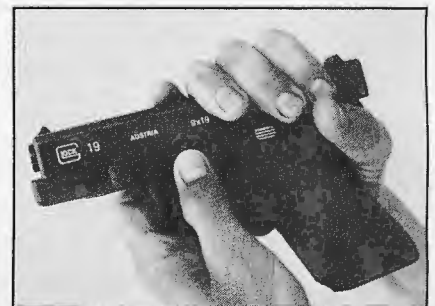
Illustrated is the correct procedure for separating the slide from the frame as explained in the text.
